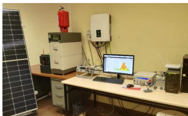
Fig. 8. Experimental \text{LiFePO}_4 Battery Cycling System. Simulation of a stand-alone/on-grid Photovoltaic applications.
