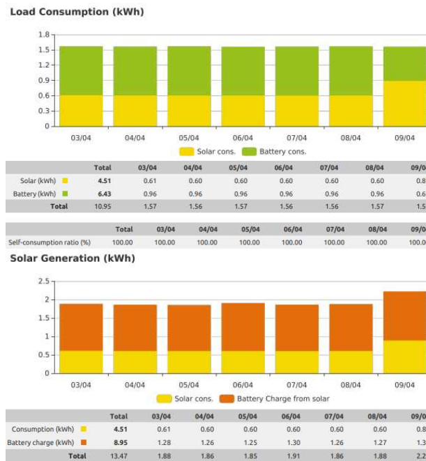
Fig. 15. Weekly report with the energy results of the stand-alone photovoltaic system with battery energy storage system.
