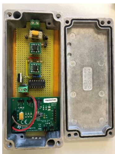
Fig. 4. Photograph of the control electronics of the EFEH system together with the DC/DC power converter.
