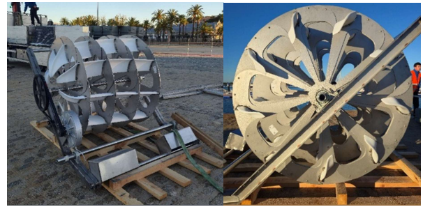
Fig.2. Kliux cross-flow hydrokinetic turbine: rotor detail (left) and blade geometry (right).
