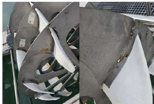
Fig. 7. Turbine blade surfaces after sustained operation, showing absence of biofouling due to continuous rotor motion.
