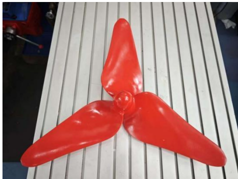
Fig. 1. Rotor designed for low-velocity conditions
