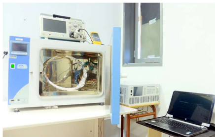
Fig. 3. Photograph of the experimental setup for determining the \delta_{eff} , \mu_{r,eff}' and \mu_{r,eff}'' for cores of the conductors Crocus 288 and 135AL1 conductors.
