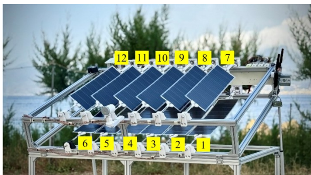
Fig. 1 Photograph of the scaled in power double-layer PV prototype.
