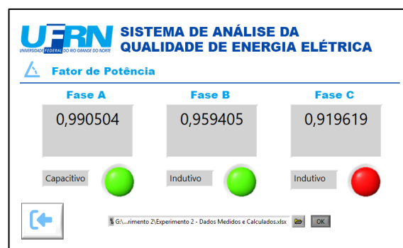
Fig. 6. Power Quality interface focusing on Power Factor analysis and compliance verification.
