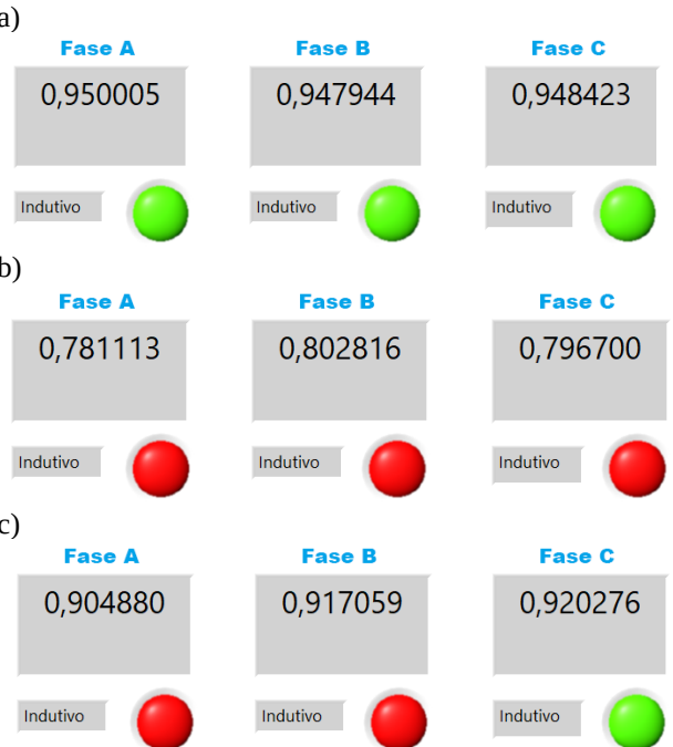
Fig. 11. Power Factor dynamics detected by the software: (a) Baseline operation; (b) Inductive load step; (c) Reactive power compensation.
