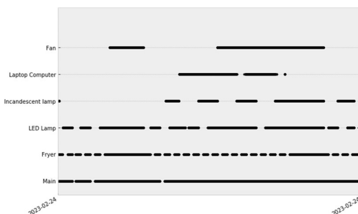
Fig. 4. Activity log for using a 10 W threshold for UALM2.
