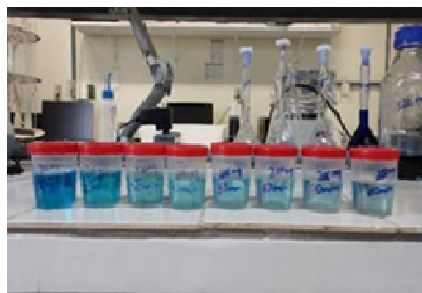
Fig.4. Methylene blue adsorption onto activated carbon produced from black wattle bark
