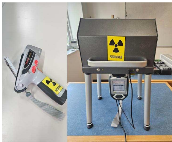
Fig. 3. Portable XRF analyzer (Niton XL3t GOLDD+) with PTS measurement stand used for stable and repeatable analysis of insulation samples
